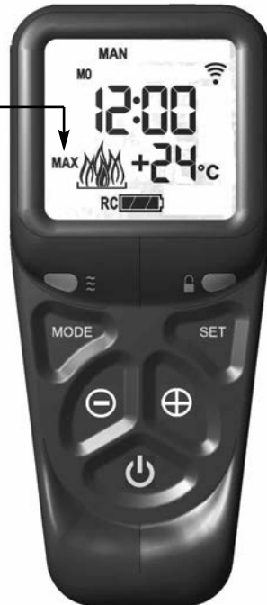
Fig. 3 - "MAX" & large flame symbol displayed
