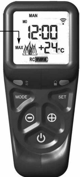
Fig. 35 - "MAX" & large flame symbol displayed
